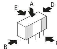
Please chuck the  portion. Avoid chucking the center of the relay. In addition, excessive chucking pressure to the pinpoint of the relay should be also avoided.
