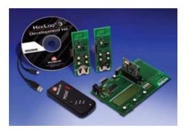
The low-cost KeeLoq 3 Development Kit is designed to help engineers get up to speed quickly using PIC® microcontrollers (MCUs), and provides everything needed to program, debug, and develop secure authentication applications for a variety of markets such as security systems (keypads, remote sensors and access control); remote keyless entry (automotive) and authentication (identity and property) applications.
