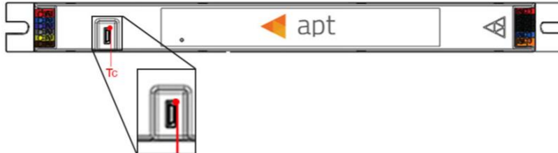
Fig. 4 - T c is measured on metal sleeve of micro-USB programming port in location specified above
