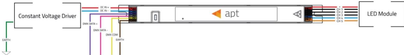
Figure 2 - APT-CV5-VA DMX512/RDM Configuration
