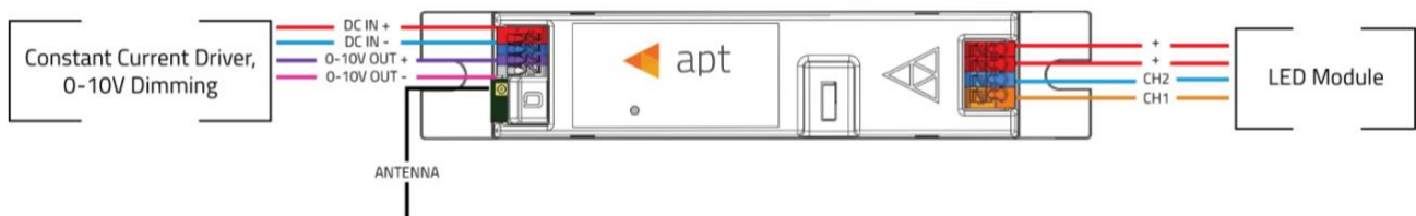
Figure 3 - APT-CC-VWx-LN Wireless Communication Configuration
