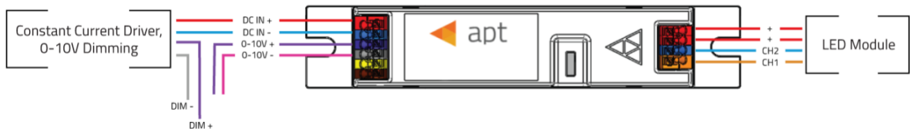
Figure 4 - APT-CC-VD-LN 0-10V Configuration
