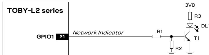
Figure 65: Application circuit for network indication provided over GPIO1
