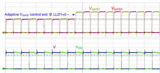
Figure 58.  $V_{GATE}$  Control Exits when LLD is Low
