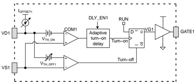
Figure 43. SR Turn-on Algorithm
