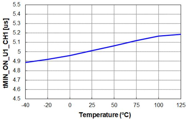
Figure 5. t<sub>MIN\_ON\_U1\_CH1</sub> vs. Temperature
