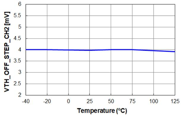
Figure 10. V<sub>TH\_OFF\_STEP\_CH2</sub> vs. Temperature
