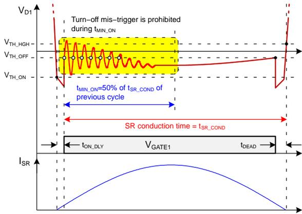
Figure 49. Minimum Turn-on Time and Turn-off Mis-triggering
