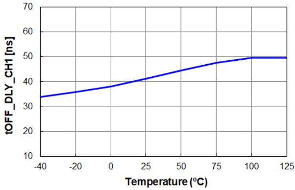
Figure 21. t<sub>OFF\_DLY\_CH1</sub> vs. Temperature
