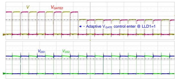
Figure 57.  $V_{GATE}$  Control Enters when LLD is High
