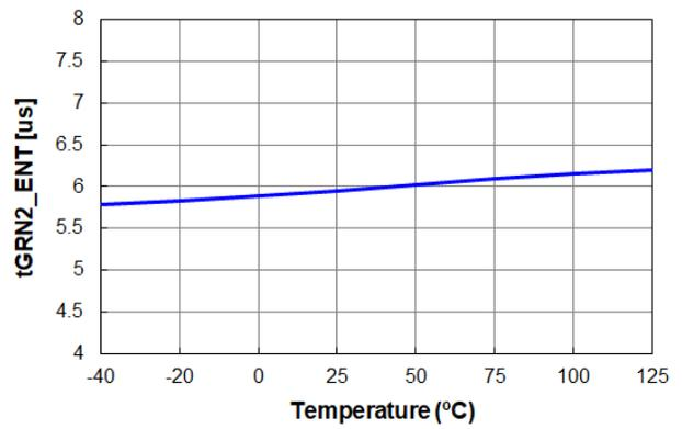
Figure 42. t<sub>GRN2\_ENT</sub> vs. Temperature
