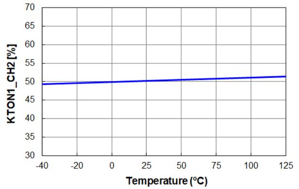
Figure 24. K<sub>TON1\_CH2</sub> vs. Temperature
