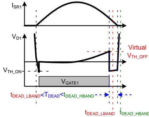
Figure 48. When  $t_{DEAD\_LBAND} < T_{DEAD} < t_{DEAD\_HBAND}$
