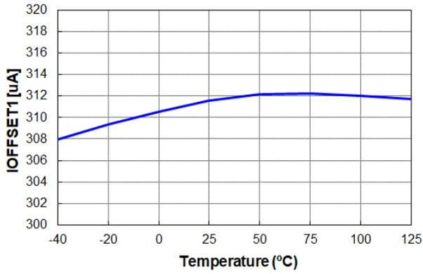
Figure 3. I<sub>OFFSET1</sub> vs. Temperature
