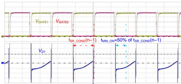
Figure 50. Minimum Turn-on Time  $t_{MIN\_ON}$  when  $DLY\_EN = 0$
