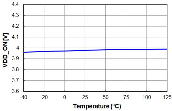
Figure 11. V<sub>DD\_ON</sub> vs. Temperature
