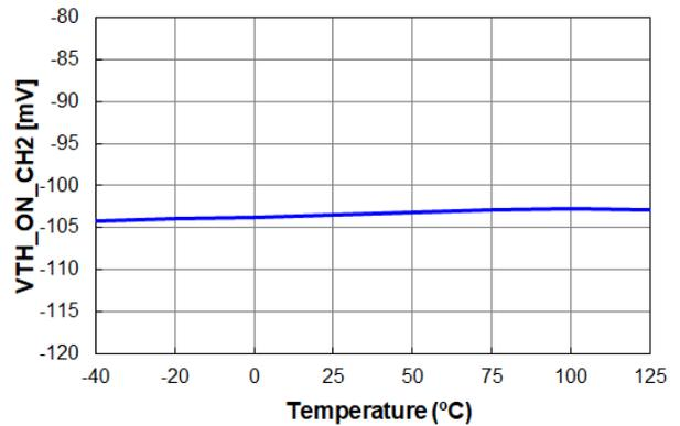
Figure 8. V<sub>TH\_ON\_CH2</sub> vs. Temperature
