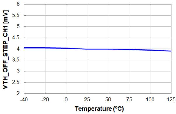
Figure 9. V<sub>TH\_OFF\_STEP\_CH1</sub> vs. Temperature
