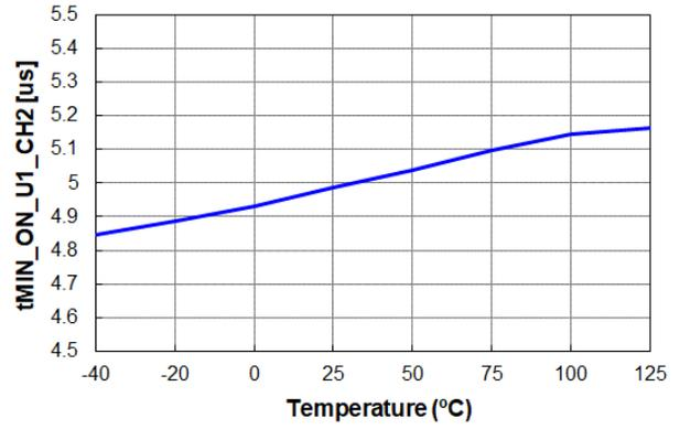
Figure 6. t<sub>MIN\_ON\_U1\_CH2</sub> vs. Temperature
