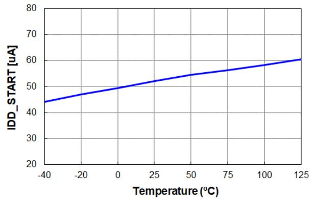
Figure 14. I<sub>DD\_START</sub> vs. Temperature
