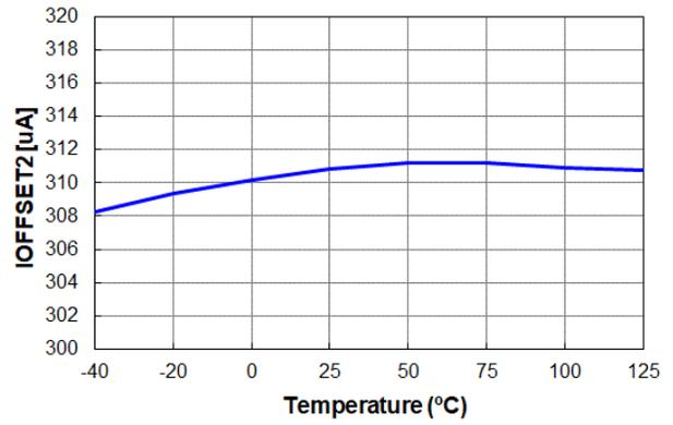
Figure 4. I<sub>OFFSET2</sub> vs. Temperature
