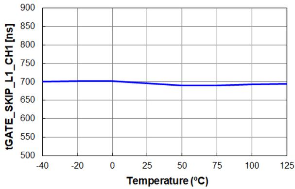
Figure 39. t<sub>GATE\_SKIP\_L1\_CH1</sub> vs. Temperature
