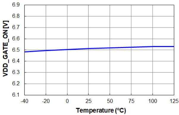
Figure 13. V<sub>DD\_GATE\_ON</sub> vs. Temperature
