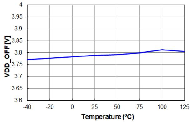
Figure 12. V<sub>DD\_OFF</sub> vs. Temperature
