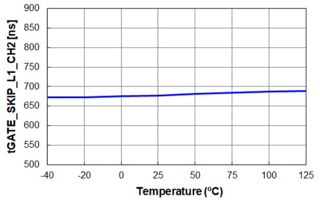
Figure 40. t<sub>GATE\_SKIP\_L1\_CH2</sub> vs. Temperature
