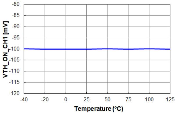
Figure 7. V<sub>TH\_ON\_CH1</sub> vs. Temperature
