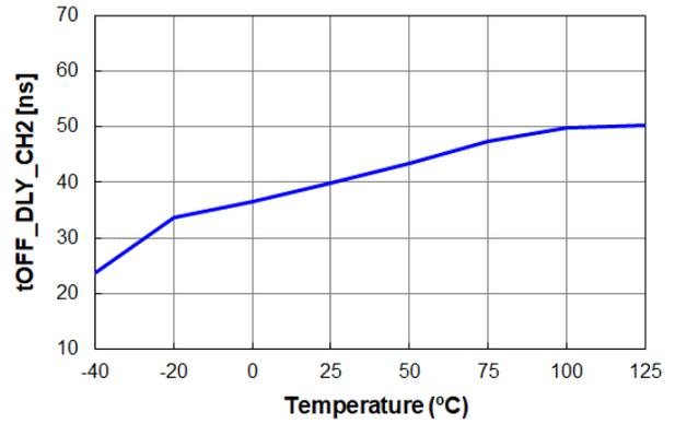
Figure 22. t<sub>OFF\_DLY\_CH2</sub> vs. Temperature
