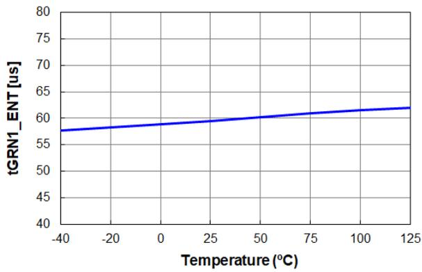
Figure 41. t<sub>GRN1\_ENT</sub> vs. Temperature
