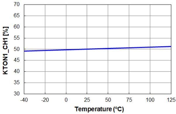
Figure 23. K<sub>TON1\_CH1</sub> vs. Temperature
