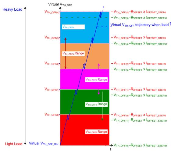
Figure 54. Virtual  $V_{TH\_OFF}$  Trajectory when Iout Increases
