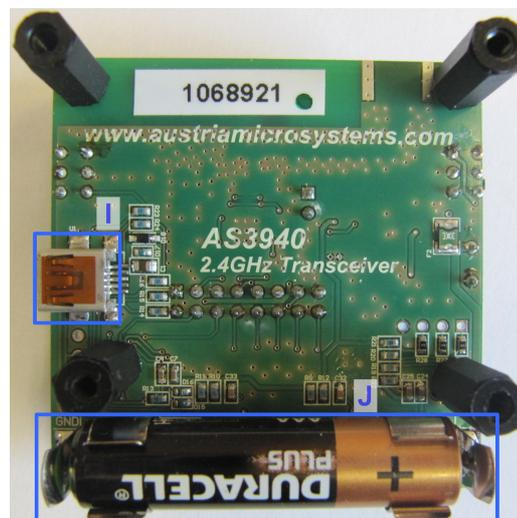
Figure 2: Board Description Bottom – Connectors
