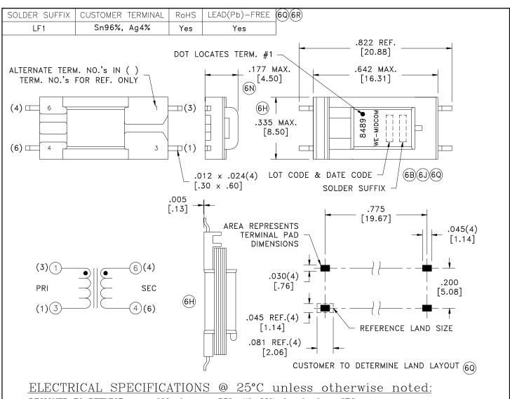
DESIGNED TO REFLECT: 600 ohms on PRI with 287 ohm load on SEC.
