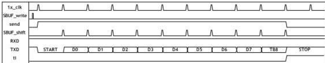
Figure 6.10 Timing Diagram for UART Transmission Mode3
