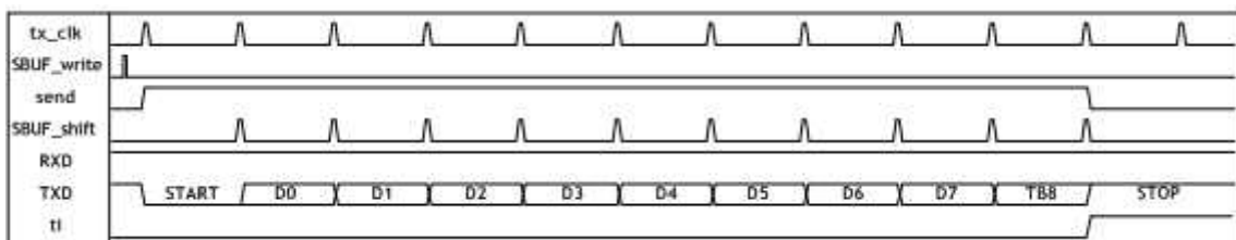
Figure 6.9 Timing Diagram for UART Transmission Mode2
