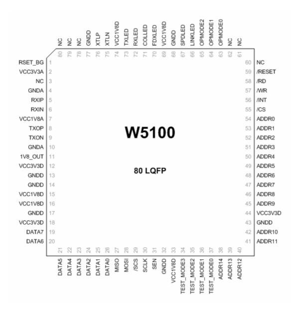
Figure 1. Pinout W5100
