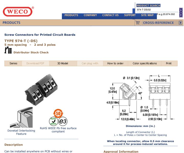
can be installed anywhere on PCB without wires or screws interfering with the rest of PCB. Can be located next to each other back-to-back, front-to-front and front-to-back. The screws and wire entries are easily visible, accessible and usable, an ergonomic advantage.
