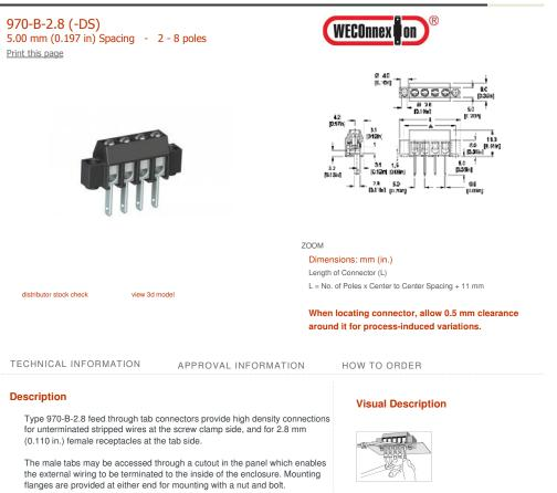
Recommended mounting hardware: M2 cheese head screw (#2-56 fillister head screw) or similar sized sheet metal screw, self-tapping screw or rivet.
