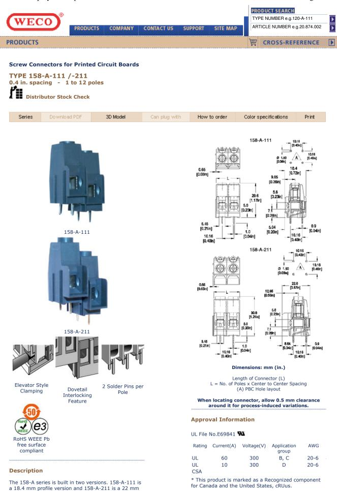
Screw Tightening Torque: UL: 11.5 lbfin Rated Impulse Withstand Voltage: 8 Kv
