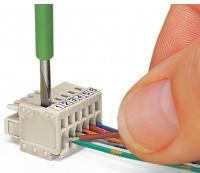
Inserting conductor via (2.5 x 0.4) mm screwdriver – CAGE CLAMP® actuation perpendicular to conductor entry.
