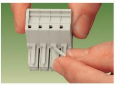
Break or cut-off coding pin on the female connector  $\ldots$
