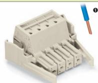
① can be connected: 0.5 mm² - 10 mm² "s + f-st"; can be pushed in directly: 1.5 mm² - 10 mm² "s" and 1.5 mm² - 6 mm² "insulated ferrule, 12 mm/0.472 in"
