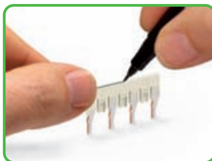
Staggered jumper 1 – 3 – 5 – 7 Marking with a felttip pen
