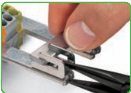
To remove the busbar, compress the spring using pliers
