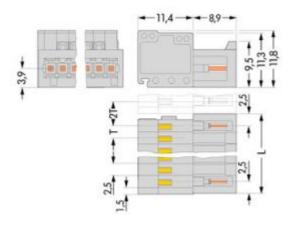
T = 2.5 mm= (No.of poles + 1) x pin spacing
