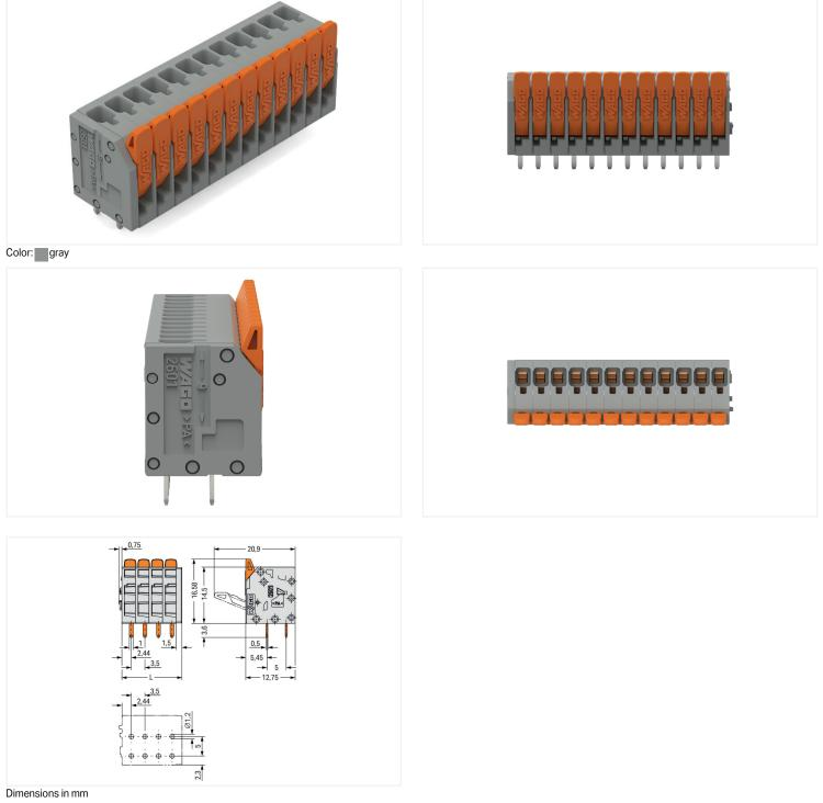
L = (pole no. -1) x pin spacing + 5 mm
