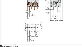
L = (pole no. -1) x pin spacing + 5 mm
