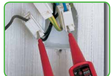
Testing through separate test slot
