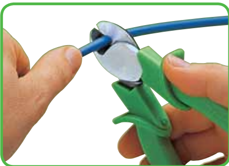
Cutting of wire
