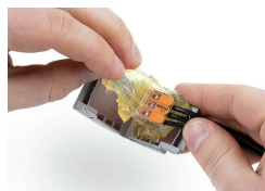
Re-accessible: Open the Gelbox. Remove the gel. Rewire with new components.
