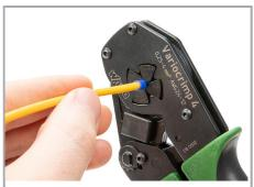
Squeeze handles until ratchet mechanism is released.
