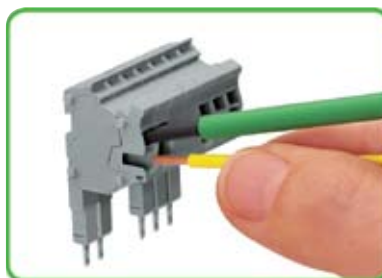
Wire connection: Screwdriver actuation for connection of all conductor types, i.e. stripped stranded conductors, or push-in connection of solid or ferruled stranded conductors.
