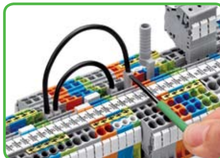
Push down the wire jumper until fully inserted. Lift the jumper with a screwdriver for rewiring.
