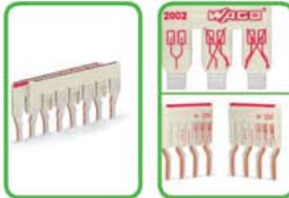
Two staggered jumpers 1 - 3 - 5 - 7 Locate red stripes of the staggered jumpers on the inside Staggered for use in a jumper slot
