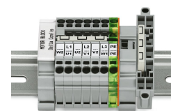
This delta jumper has been specially developed to create a delta configuration and is used on motor terminal boards equipped with rail-mount terminal blocks TOPJOB® S.
