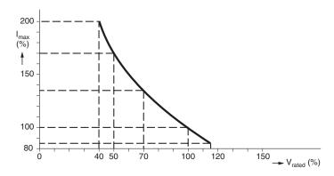
I<sub>max</sub> as stated in the Electrical data and ordering information tables, is the maximum overload current that may flow through the PTC when passing from the low ohmic to high ohmic state at rated voltage.
