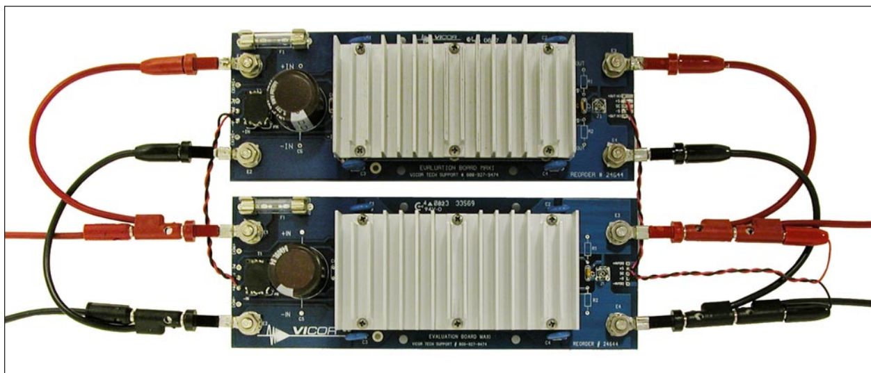
Figure 6: Paralleled Evaluation Board, wire gage is suitable for high input and output voltage converters
