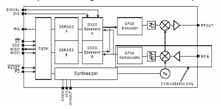
Figure 2 – Radio Simplified Block Diagram
