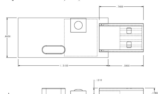
Figure 4 - Juno-USB Dimensions (internal)
