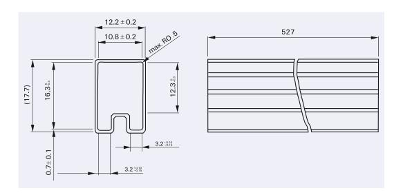
Tube for THT version 25 relays per stick 1'000 relays per box
