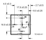
For the make conta87(2937), pin 87a = 87; for the double make contact, pin 87a = 87b. Mounting hole layout (bottom view)
