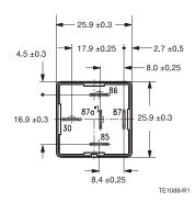
For the make contact (2x87), pin 87a = 87; for the double make contact, pin 87a = 87b.
