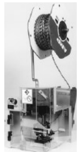
Entry Level Terminator (Requires Applicators and Dies)
