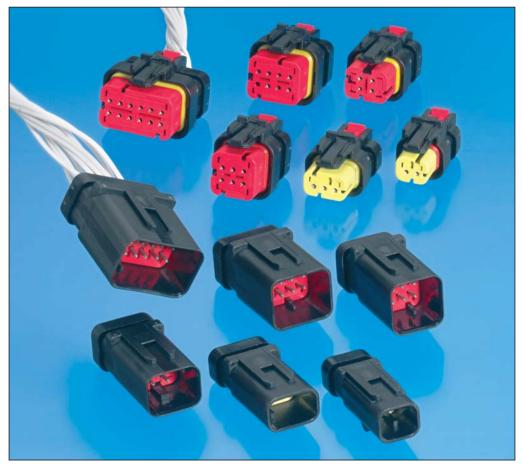
The AMPSEAL 16 Receptacle and Pin housings come fully assembled, offering a one-piece approach for applied cost savings. Receptacle housing assemblies consist of the plug housing with both interface and wire seals, wire seal cover, PLR & CPA.
