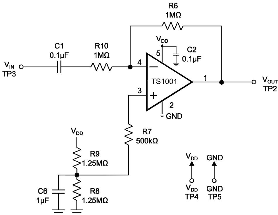
Figure 2. Inverting Configuration
