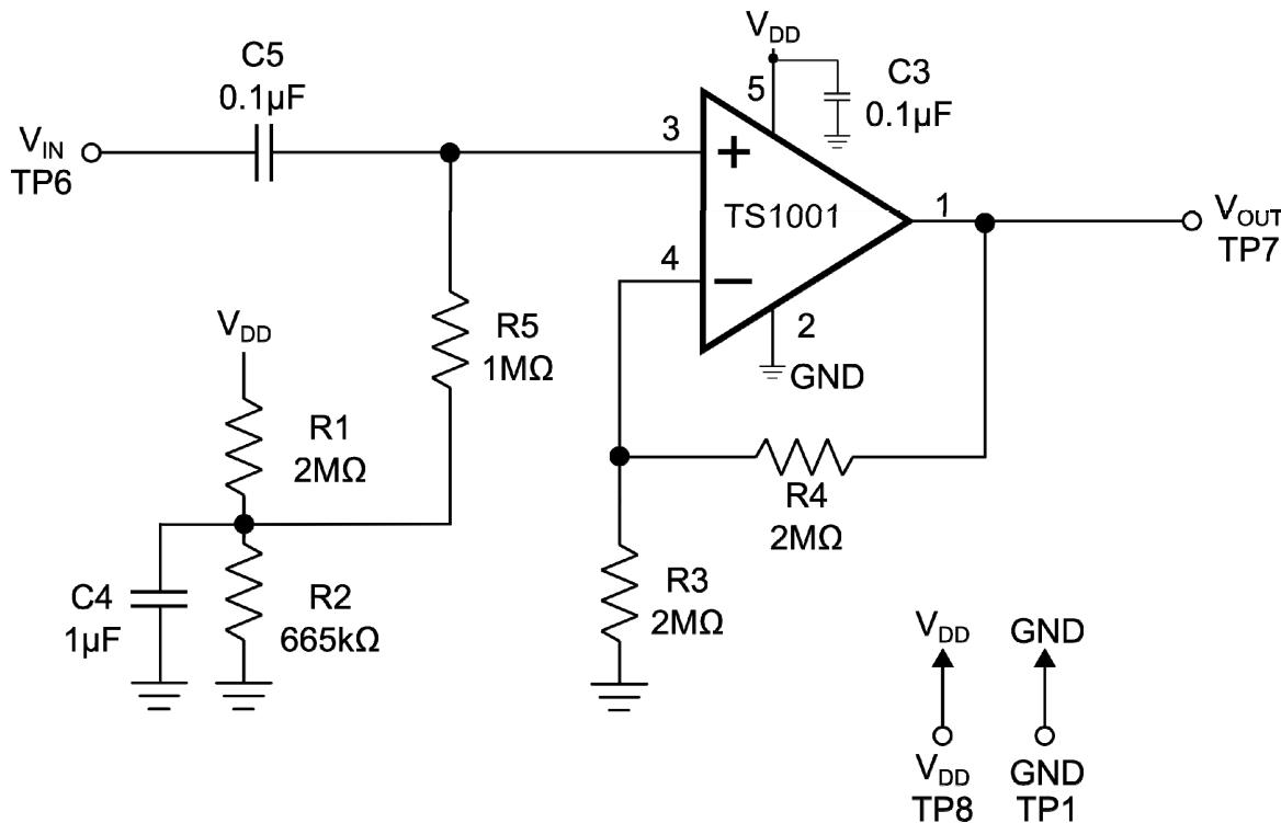
Figure 1. Non-Inverting Configuration
