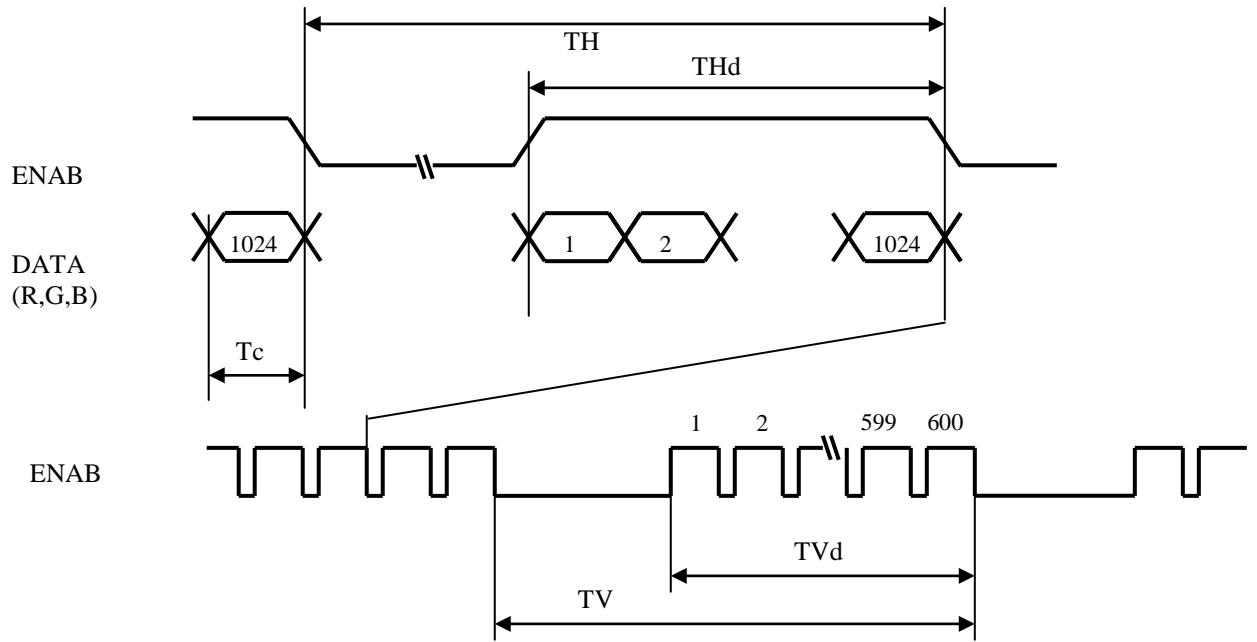
7 - 2. Input data signals and display position on the screen
