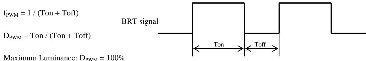
In case of using the low frequency, the deterioration of display quality, flicker, etc, may occur.
