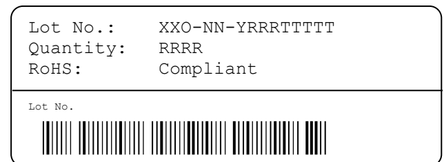
Figure 22: First label on reel: XX = Sensor Type (25 for SHT25), O = Output mode (D = Digital), NN = product revision no., Y = last digit of year, RRR = number of sensors on reel divided by 10 (200 for 2000 units), TTTT = Traceability Code.
