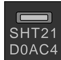
Figure 21 Laser marking on SHT21. For details see text.
