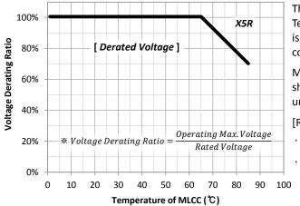
\* Temperature of MLCC : Surface temperature of MLCC in the circuit.
