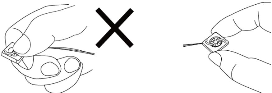
**Don't pull fan with lead wires.**
