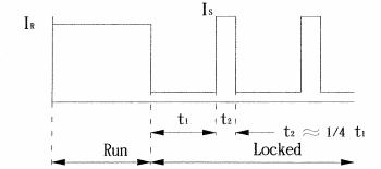
3rd wire signal Run : Square Wave Locked : VH or VL
