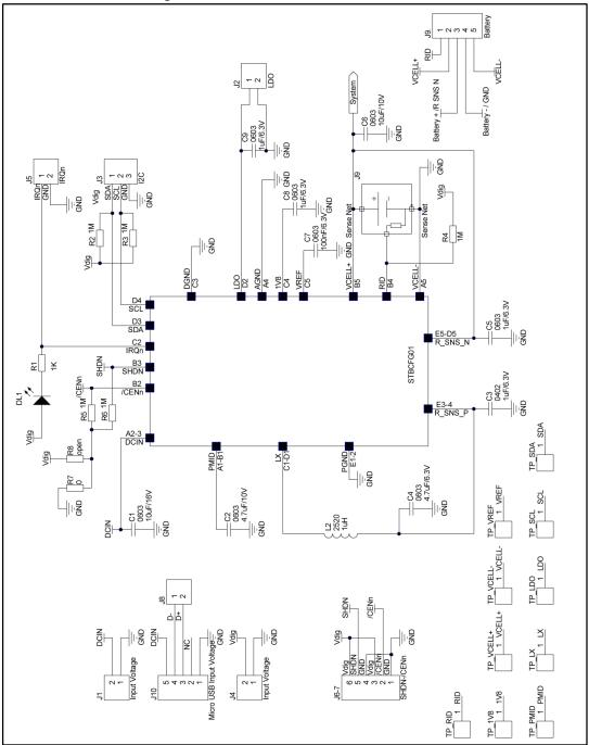
Figure 1: STEVAL-ISB033V1 circuit schematic
