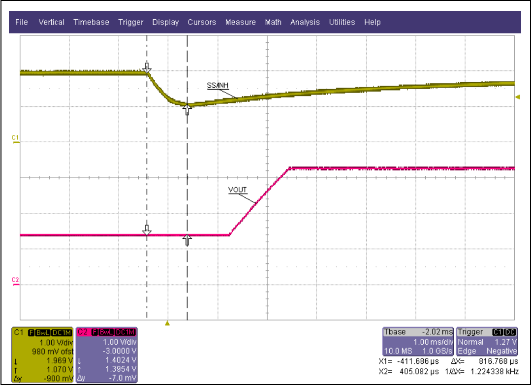
Figure 9. External soft-start after UVLO or thermal shutdown
