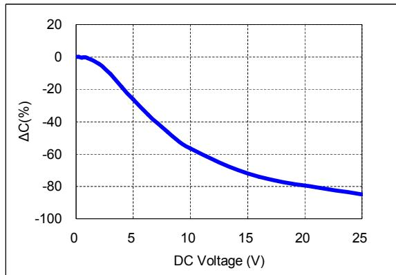
4) Bias TCC characteristics (Agilent 4284A, 120Hz, 0.5Vrms, 12.5Vdc)
