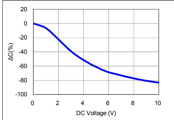
4) Bias TCC characteristics (Agilent 4284A, 1kHz, 0.5Vr, 5Vdc)
