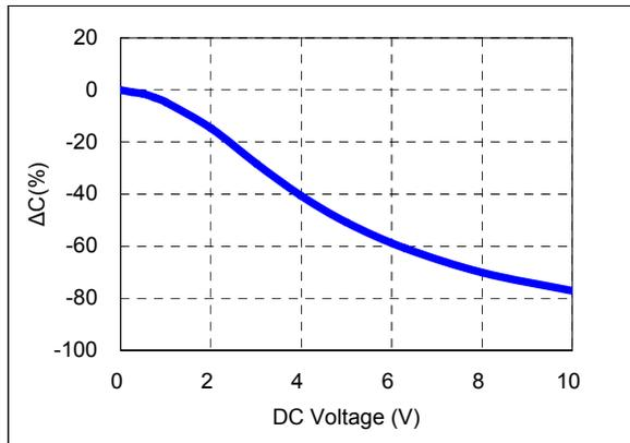
4) Bias TCC characteristics (Agilent 4284A, 1kHz, 1Vrms, 5Vdc)
