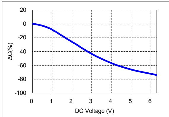
4) Bias TCC characteristics (Agilent 4284A, 1kHz, 1Vrms, 2Vdc)
