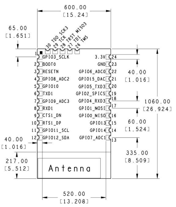
NOTE: An antenna area of 217X520 mils need to be free of any ground metallization or traces under the unit. The area extending away from the antenna should be free from metal on the PCB and housing to meet expected performance. Pin 25 is the required paddle ground and is not shown in this diagram.
