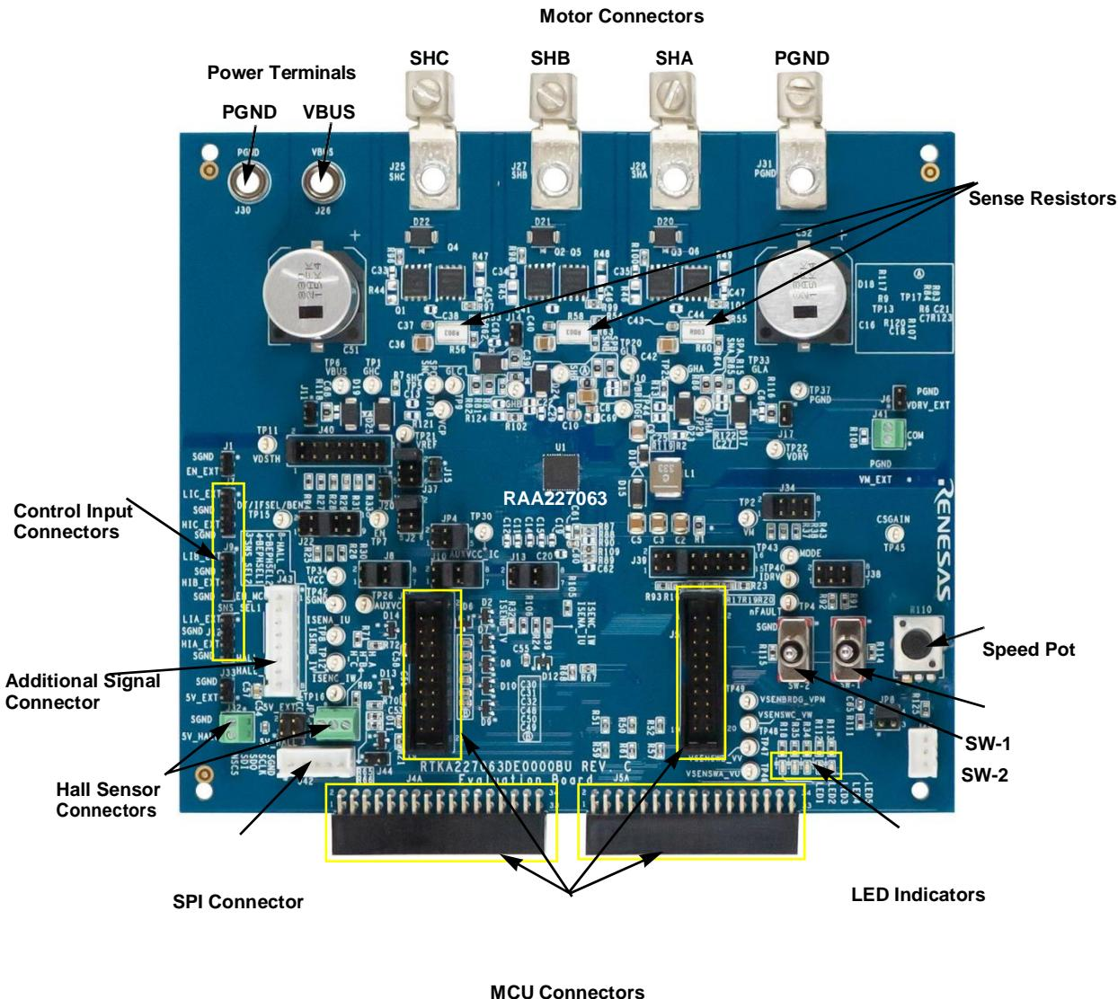
Figure 2. RTKA227063DE0000BU Evaluation Board (Top View)
