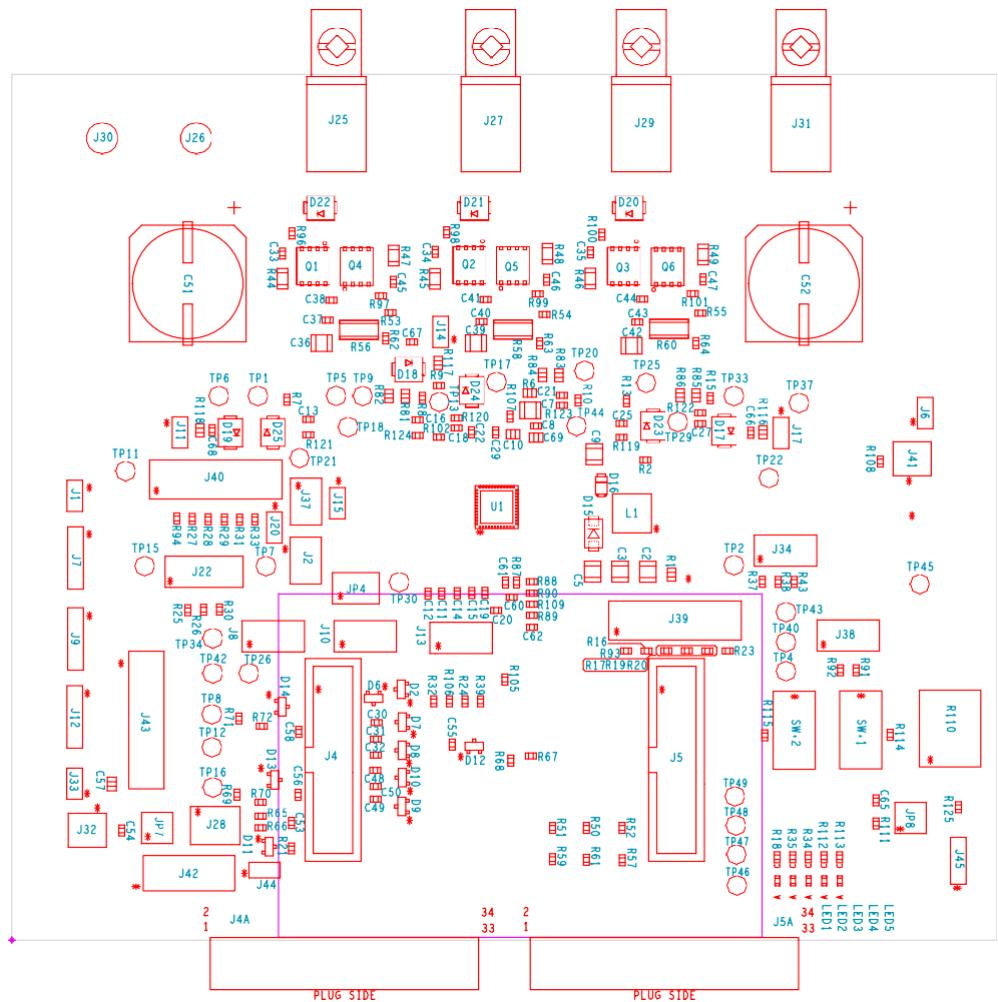
**Figure 12. Evaluation Board Assembly Top**
