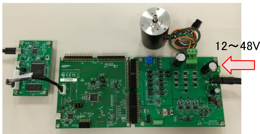
Figure 4-10 Power supply from DC jack
