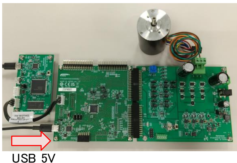
Figure 4-12 Power supply from USB connector
