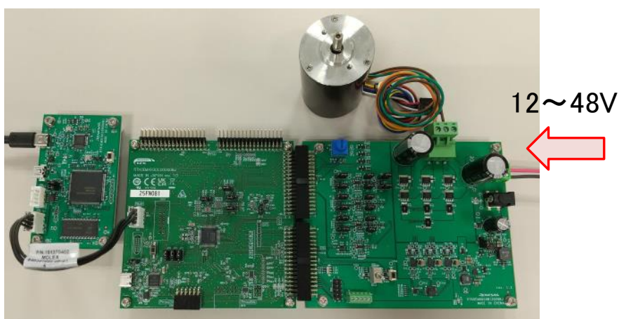
Figure 4-11 Power supply from terminal block
