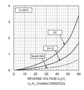
REVERSE POWER DISSIPATION:P<sub>R</sub>(W)
