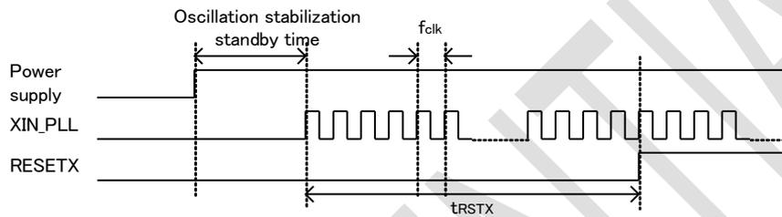
Figure V.1 Reset Timing
