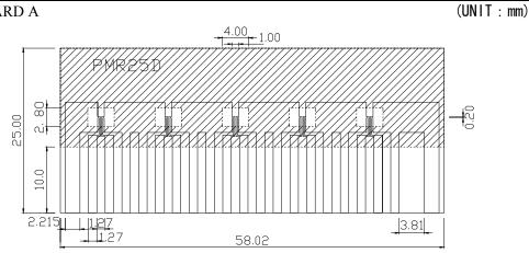
NOTE) \*1 The shaded area shows the solder resist treatment.
