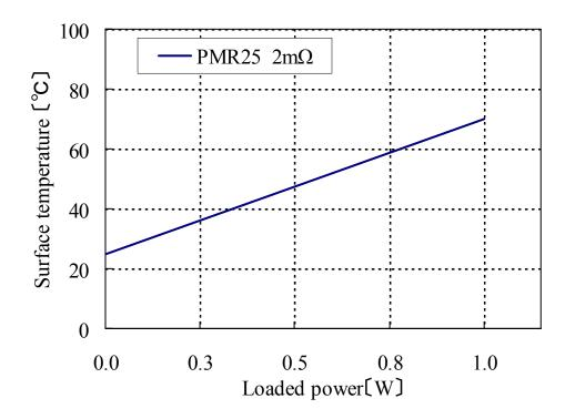
(Note) The above data is measured by the company and only for reference. The surface temperature could be effected not only by the loaded power but by the type of mounting board material, the wiring pattern, heat dissipation from the surrounding components and ambient temperature.
